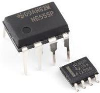
The 555 Timer has been the work horse for generating timed voltage pulses since 1971<sup>2</sup>. Add a few resistors and capacitors to get pulse widths and pulse rates over a wide range. However, longer than a few seconds starts to sacrifice accuracy and above a minute demands special capacitors.
